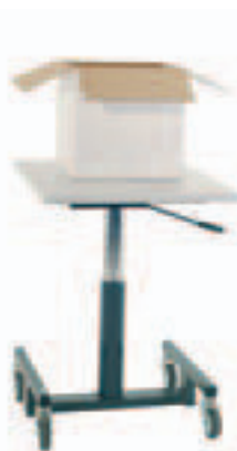
Packing and commissioning trolley for the simple filling of different-sized boxes. The pneumatic jack enables the operator to lift full cartons (max. 30 kg) up to table height with ease.
